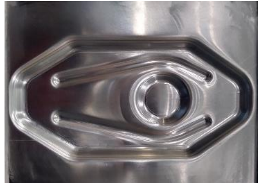
Base die – Two-Point Incremental Forming Strategy
